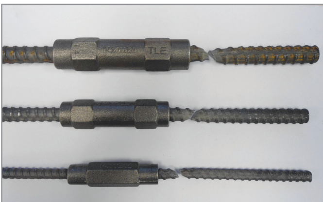
F47 Threaded Bar couplers will develop the full breaking strength of the bar
